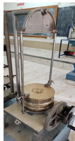
Fig 4.5: screening of fly ash
