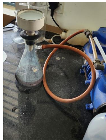
Fig 4.3: Vacuum filtration of modified fly ash
