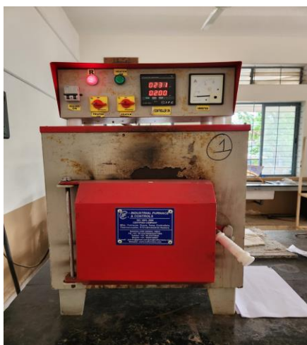
Fig 4.4: Drying in muffle furnace
