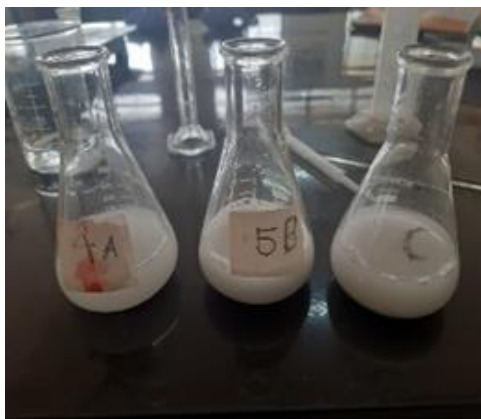
Fig 4.6: Flask containing stock solution and fly ash
