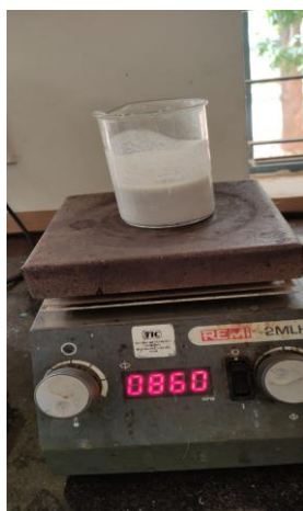
Fig 4.2: Agitation of fly ash with modifier solution
