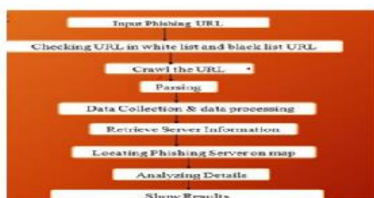
Fig 2 Flow Diagram of content based approach
