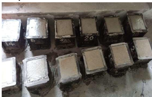
Fig 3. Preparation of moulds
