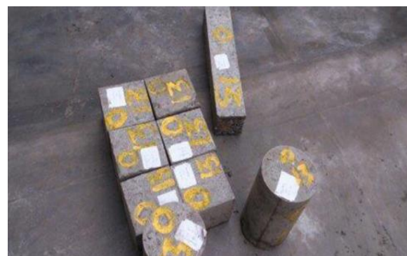
Fig 3 Specimens after demoulding
