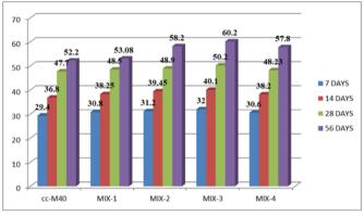
Split tensile strength of concrete with mix design of M40
