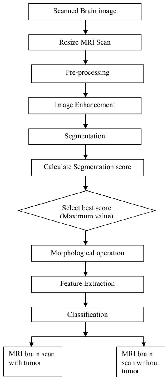
Fig. 1 Block diagram of MRI Brain tumor image methodology for detection and classification
